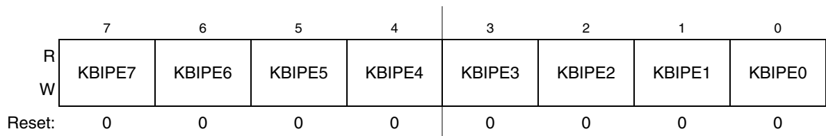
Figure 10-4. KBI Pin Enable Register
